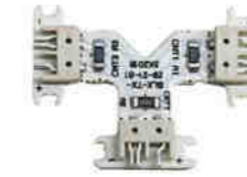
42AA06EL 3 ways electrified connector.
